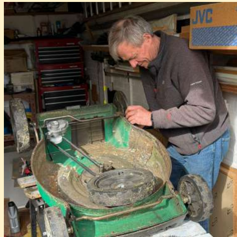
Reassembly with new gear box/clutch and belt
