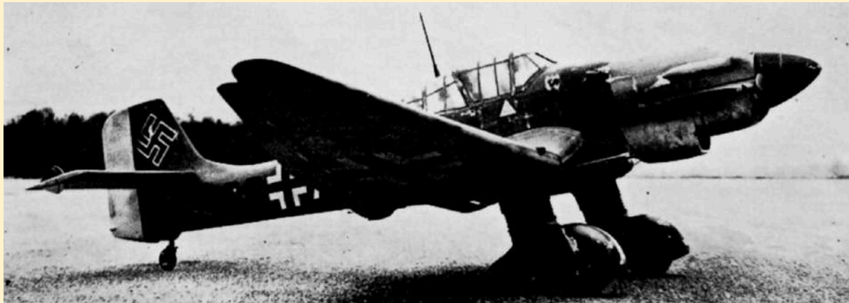
Only the small propeller gives the Stuka away as not being the real thing. Glass fibre wheel pants have concertina trouser effect incorporated. Ailerons are full span with differential.
